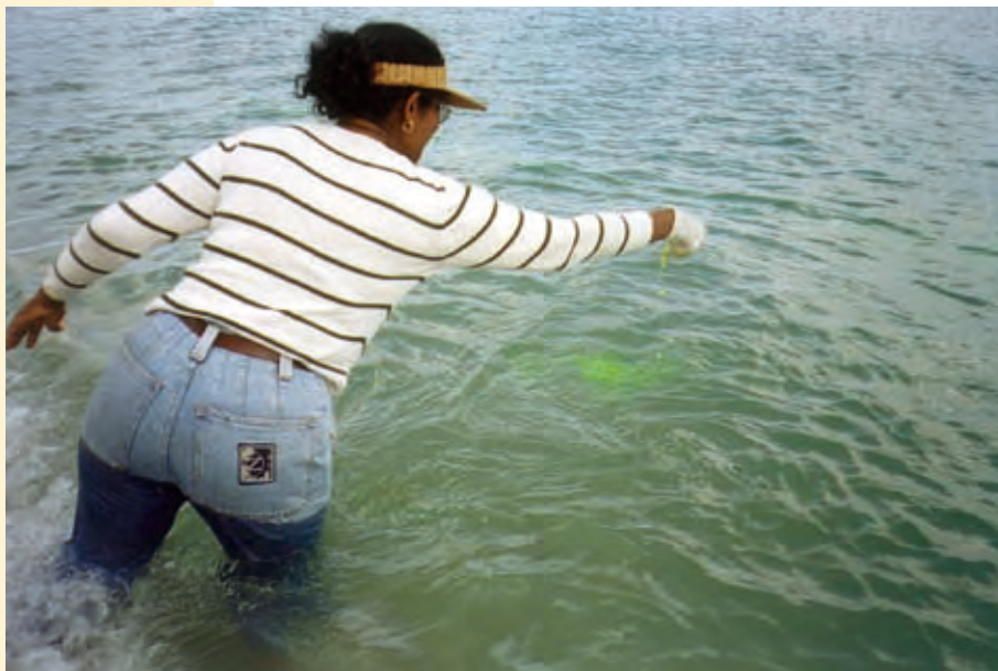
Measuring longshore currents with fluorescent dye.
