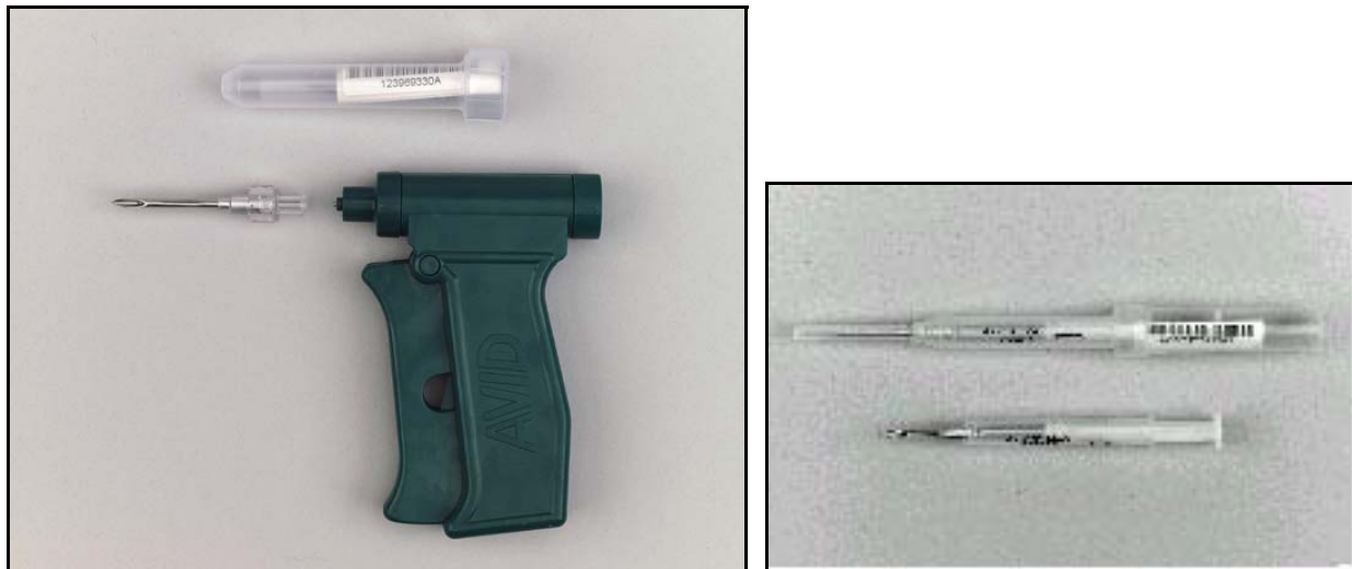
Figure 4. Tag delivery systems vary, even within manufacturers (in this case, AVID). The Disposable Needle Assembly (DNA) (left) is a sterile preloaded needle assembly designed to snap into the DNA applicator gun. The Single Use Disposable Syringe (SUDS) (right) is a sterile syringe pre-loaded with the PIT tag (microchip). The protective cover is snapped off prior to injection. (Note: SUDS is arguably the simplest method, but it produces a lot of waste because components are used only once.) Source: http://www.ezidavid.com/prod01.htm
