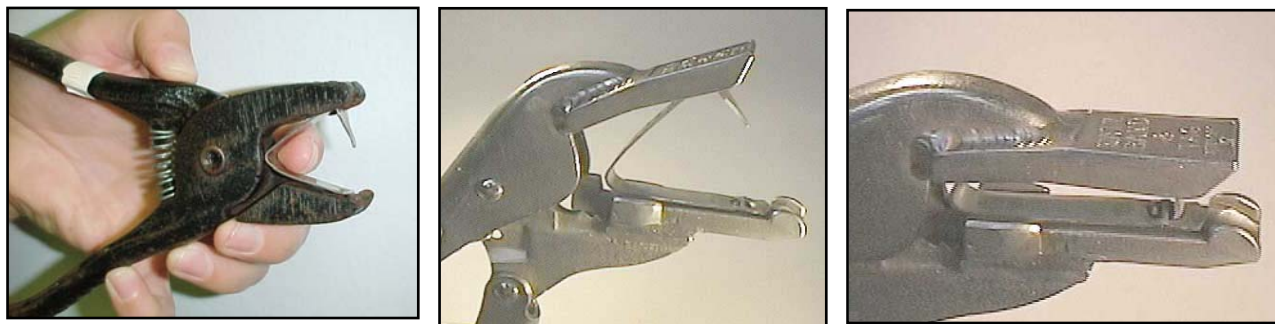
Figure 8. A Monel 1005-49 style metal flipper tag correctly loaded (left) and cinched (right) in the application pliers. ALWAYS align the base plate of the tag flat against the pliers. Note the tine bent over and completely through the stirrup. Source: http://www.nationalband.com/nbt.pdf
