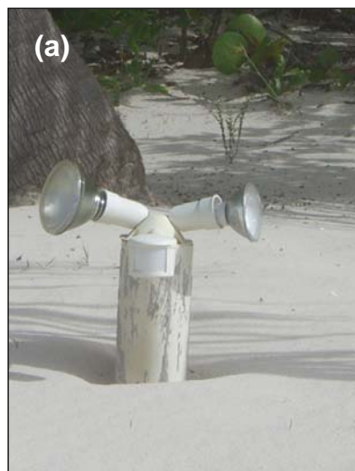
(a) Low, pole-mounted double spotlight with motion sensor (b) Activated by a motion sensor, a spotlight illuminates the beach
