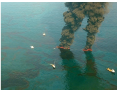
Figure 4.10. In-situ burning operations in the Gulf of Mexico during Deepwater Horizon spill in 2010. Photo: Chief Petty Officer John Kepsimelis, U.S. Coast Guard.
