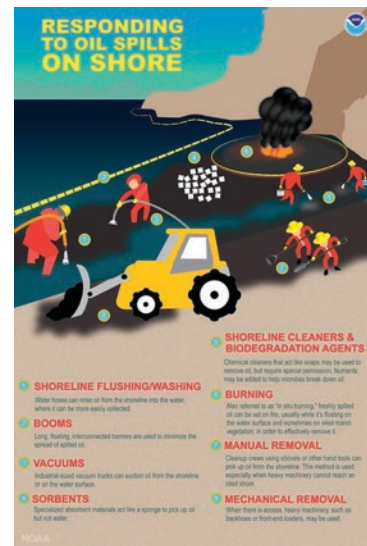
Figure 4.15. Primary response approaches for shorelines. Graphic by NOAA.
