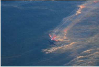
Figure 4.9. Aerial dispersant application from a Basler BT-67 fixed wing aircraft during Deepwater Horizon spill, May 2010. Photo: Petty Officer 3rd Class Stephen Lehmann, U.S. Coast Guard.
