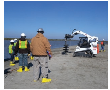
Figure 4.17. Mechanized excavation of a sand beach for SCAT during the Deepwater Horizon spill to survey for buried oil. Source: NOAA.
