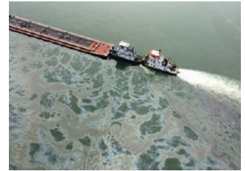
Figure 5.36. Kirby Barge 27706, loaded with marine fuel oil and partially submerged in the Houston Ship Channel, March 22, 2014. The bulk carrier Summer Wind collided with the barge, containing 924,000 gallons of fuel oil. Photo: U.S. Coast Guard.
