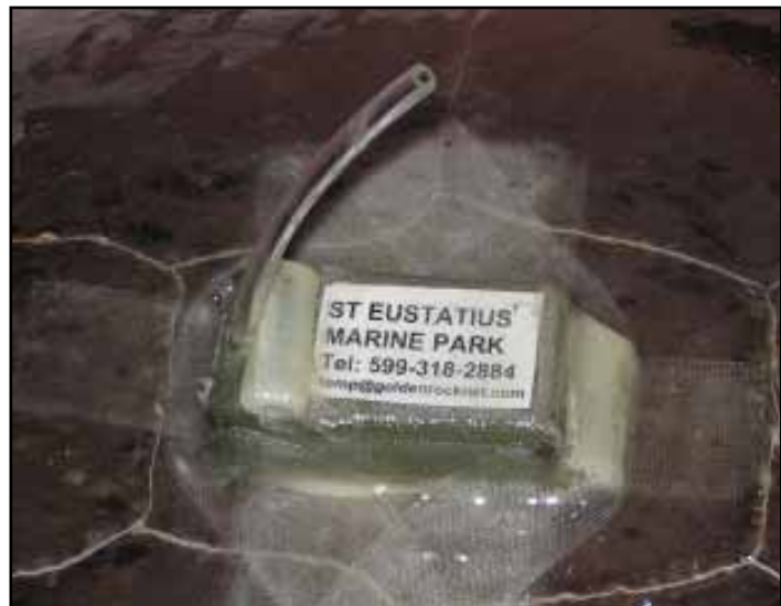
Figure 9. Satellite transmitter fitted to a turtle carapace
